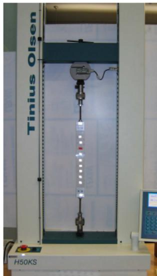
*A simple experimental set-up for a beam with clamped-pinned boundary conditions in a displacement-controlled testing machine.*
