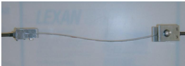
*The mode shapes corresponding to (a) the lowest natural frequency, and (b) the elastic critical load, for a clamped-pinned axially-loaded beam.*
